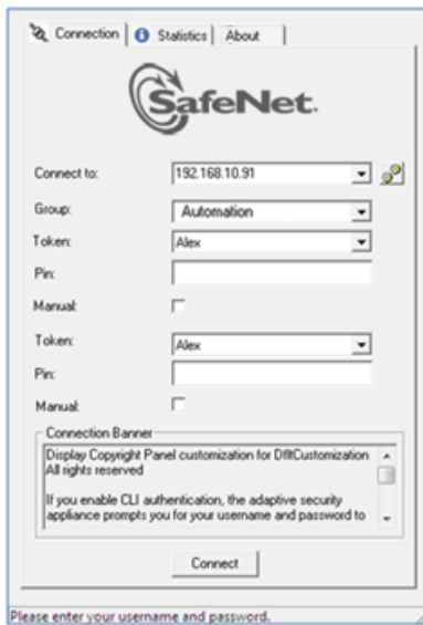
Figure 5: MobilePASS Token detection in both the Primary and Secondary Password fields
